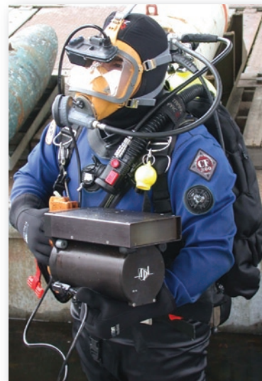
The DIDSON can be used by divers to perform security sweeps. A commercial binocular, color display interfaces with the camera and produces a large virtual image at a comfortable viewing distance.
