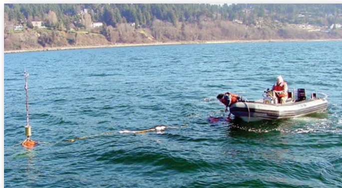
Receiving array recovery in Puget Sound. The radio frequency antenna is at the left and the battery pack is near the boat.
