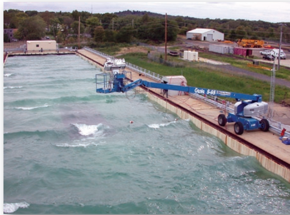
AIRS scientists participated in the Polarimetric Emissivity of Whitecaps Experiment (POEWEX) at the OHMSETT wave basin at Naval Weapons Station Earle. During POEWEX AIRS scientists used a lift crane to mount three fully polarimetric microwave radiometers above the wave basin. Waves were made to break at a fixed location so that measurements could be taken of fractional area foam coverage in the radiometer footprint, aqueous-phase turbulence, void fraction, wave height, water surface roughness, and bubble size spectra.
