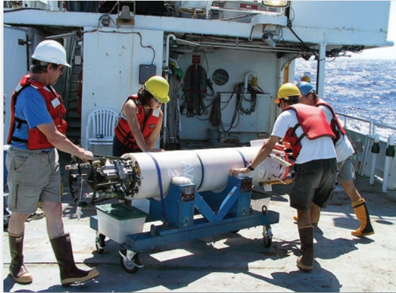
An Ocean Physics Department team prepares the Absolute Velocity Profiler for deployment.
