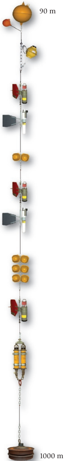
Three APL-UW-designed moorings were deployed in the Chukchi Borderland region at the beginning of the research cruise and retrieved five weeks later at the end.
